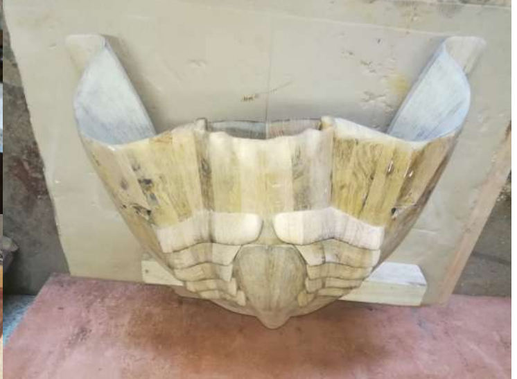
The stages of making the gills under the seat: assembly using mortise and tenon technique, the sculpted gills, and the final result.
