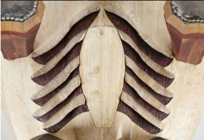
The stages of making the gills under the seat: assembly using mortise and tenon technique, the sculpted gills, and the final result.
